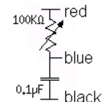
Small changes in the 30° rotation angle per picture can be achieved by adjusting the trimmer in the modified pan servo. You can stop the servo rotation if necessary by unplugging it!
