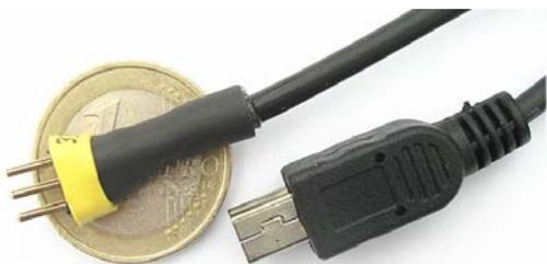
clickPAN-USB combines automatic shutter release and camera pan in one package. Comes in 2 versions for compatible Ricoh and Canon cameras. Build a light rig, without radio control, that automatically takes pictures (4 to 35 secs) &
