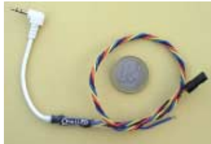
The gentLED focus. Allows control of focus AND shutter on cameras with electrical contacts.
