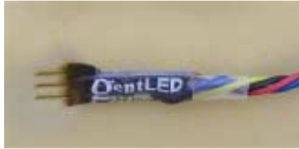
The gentLED switch. Allows control of cameras and other devices with electrical contacts.
