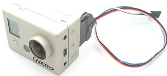
The gentWIRE-HERO. Allows control of stills or video capture with compatible GoPro cameras.
